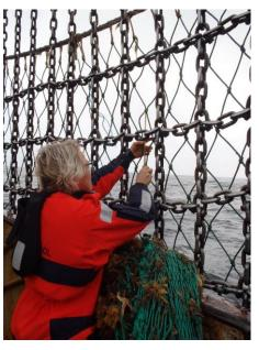
Measuring the mesh size on a beamtrawler in the North Sea.
